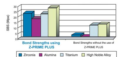
Shear Bond Strength of Z-PRIME PLUS with DUO-LINK™ (S/C) on different substrates.
