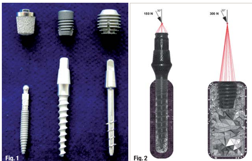
Fig. 2 _Loading direction of the numerical models. A mini implant (2.5 x 15 mm) inserted in an idealised bone block with a cortical thickness of 1.2 mm (left) and a short implant (5.5 x 7 mm) inserted in an idealised bone block with a cortical thickness of 0.5 mm (right).
