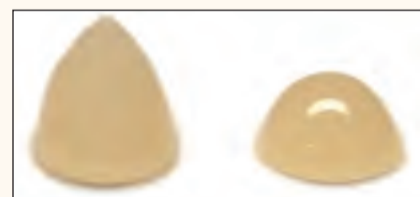
Fig. 4: "Foo" Zero Flow (0.0 mm of flow held vertically for one minute), left, is ideal for stacking, especially in the marginal ridge. "Fo3" Low Flow (3 mm of flow held vertically for one minute), right, handles more like a traditional base or liner.
