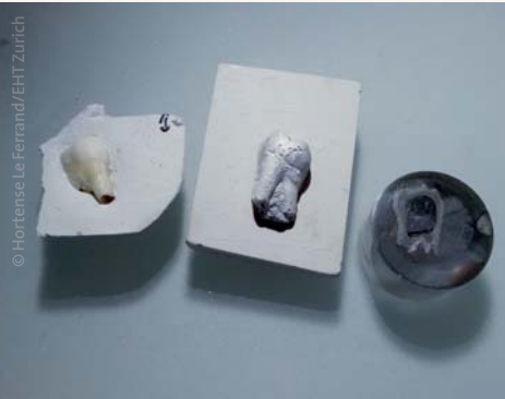
Natural tooth in its gypsum mold, artificial tooth (sintered but not yet polymer infiltrated), finished artificial tooth embedded in a “puck” to enable polishing.
