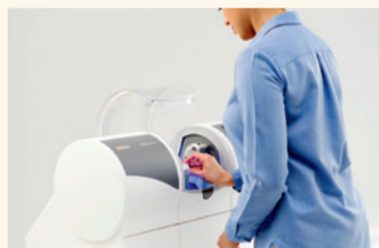
Milling: Zirconium oxide is milled in enlarged form. This allows for more detailed finishing of the structures (10 min)
