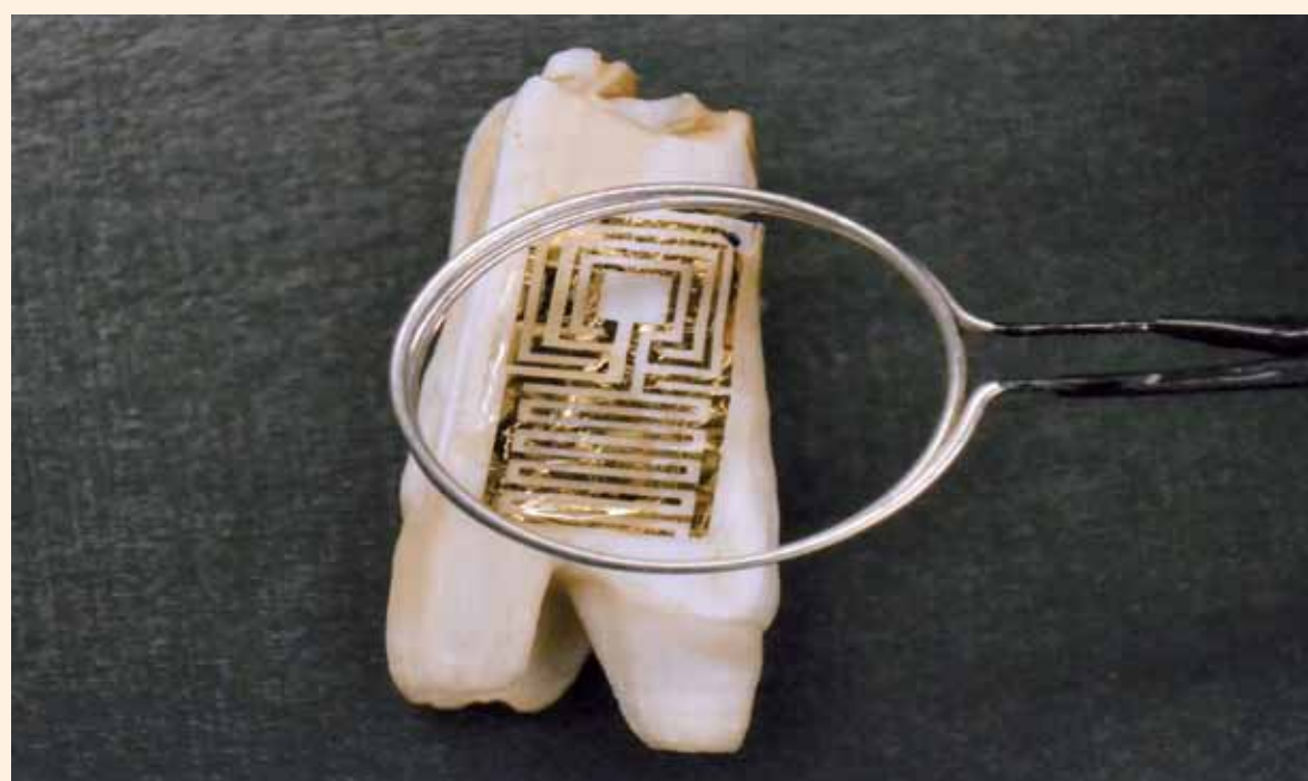
The sensor consists of a graphene layer printed on to a bioresorbable silk substrate. (DTI/Photo Princeton University, USA)
