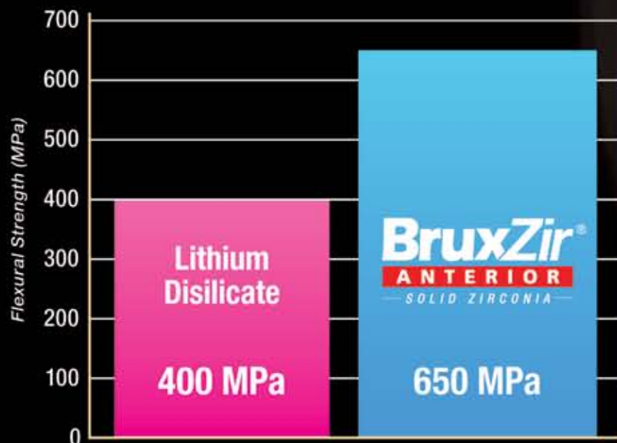
Flexural Strength Testing per ISO 6872 specification
