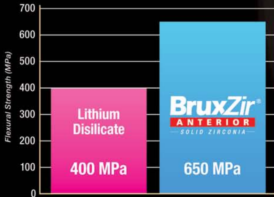
Flexural Strength Testing per ISO 6872 specification
