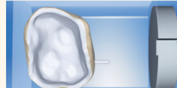
4. In the preview, I checked the position of the crown in the ceramic block. Adjustments could be made at this point if needed
