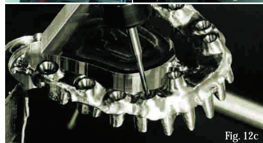
Figs. 12a-c Machining from a titanium block.
