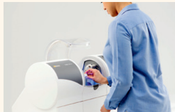
Milling: Zirconium oxide is milled in enlarged form. This allows for more detailed finishing of the structures (10 min)
