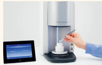
Sintering: The assistant places the restoration in the CEREC SpeedFire furnace and starts the sintering process with a touch-pad (16 min)
