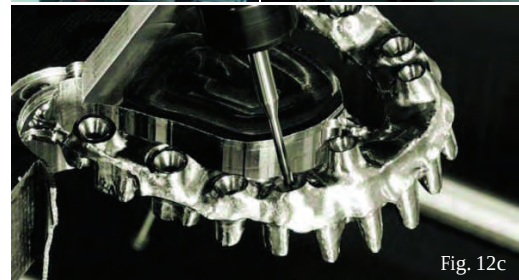
Figs. 12a-c Machining from a titanium block.
