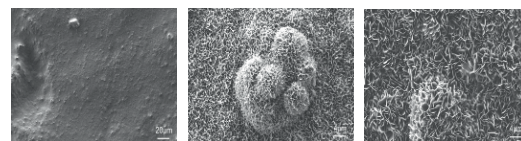
Left: Predicta Control, no SBF. Center: Predicta, 7 days in SBF. Right: Predicta, 28 days in SBF. SEM images courtesy of Håkan Engqvist, Uppsala University, Sweden.
