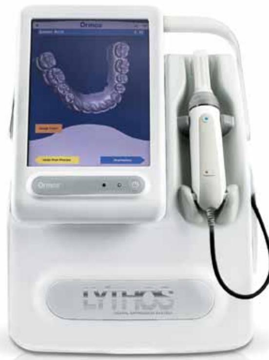
Lythos Digital Impression System can provide up to 2.5 million 3-D data points per second for a more exact and personal, single high-resolution scan.
