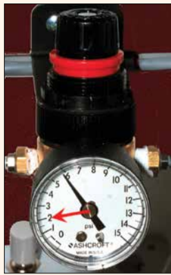
Fig. 7. The Chapman-Huffman in-line air regulator and 0-15 psi gauge works well.
