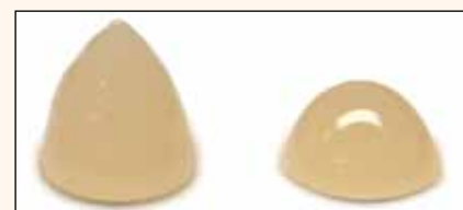
Fig. 4: 'F00' Zero Flow (0.0 mm of flow held vertically for one minute), left, is ideal for stacking, especially in the marginal ridge. 'F03' Low Flow (3 mm of flow held vertically for one minute), right, handles more like a traditional base or liner.
