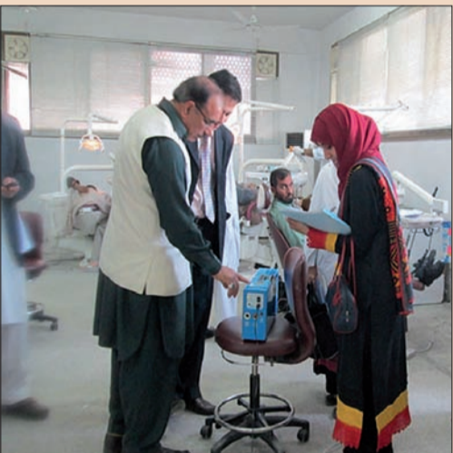
A SDPI monitoring team testing mercury levels with a Lumex Mercury Analyser in a dental clinic. (DTI/Photo courtesy of SDPI, Pakistan)
