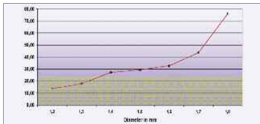
Fig. 6: The stress resistance (fracture level in Ncm) depends on the diameter of the miniscrew (according to Kyung, modification by the authors).
