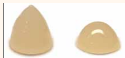
Fig. 4: "F00" Zero Flow (0.0 mm of flow held vertically for one minute), left, is ideal for stacking, especially in the marginal ridge. "F03" Low Flow (3 mm of flow held vertically for one minute), right, handles more like a traditional base or liner.
