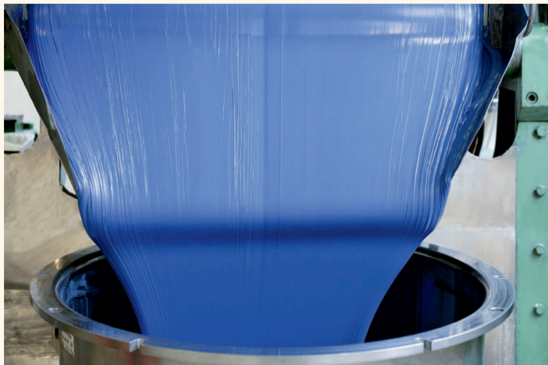
Fig. 1: Decanting of the base paste of 3M™ Impregum™ Super Quick Polyether Impression Material into a storage container.
