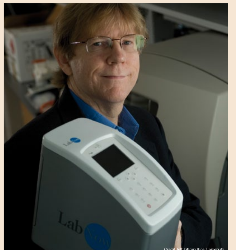
Rice University Professor John McDevitt holds the LabNow device to read nano-bio-chips that will look for signs of oral cancer and other diseases
