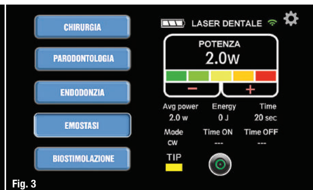
Fig. 2: The settings of the 980nm diode laser used with single-use fibres. Fig. 3: The laser settings for completely drying the sulcus with a programme in continuous-wave mode.
