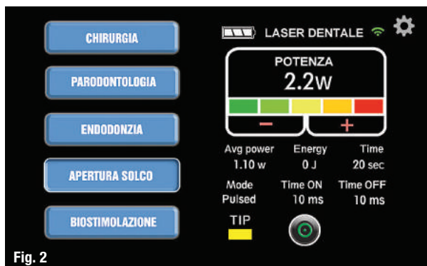
Fig. 2: The settings of the 980nm diode laser used with single-use fibres. Fig. 3: The laser settings for completely drying the sulcus with a programme in continuous-wave mode.
