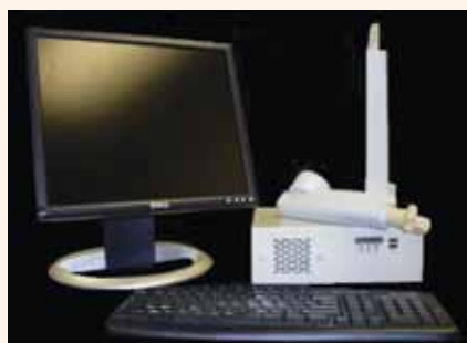
Fig. 3: A pharyngometer. (Photo/Provided by Sleep Group Solutions)
