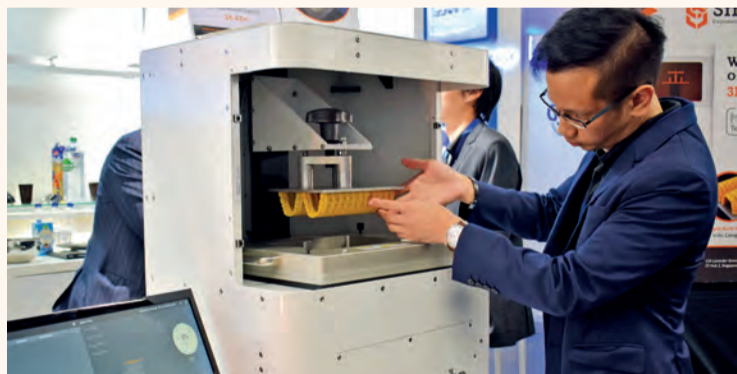
The Structo OrthoForm presented at the 2017 International Dental Show. The device is the first dentistry-specific 3-D printer tailored for orthodontic applications. ► BUSINESS Page 4
