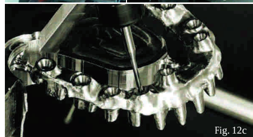
Figs. 12a-c Machining from a titanium block.
