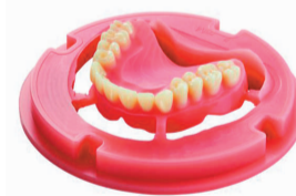
Fig 12: BDLoad, after milling process.
