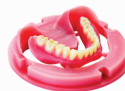
Fig 11: BDLoad, after milling process.
