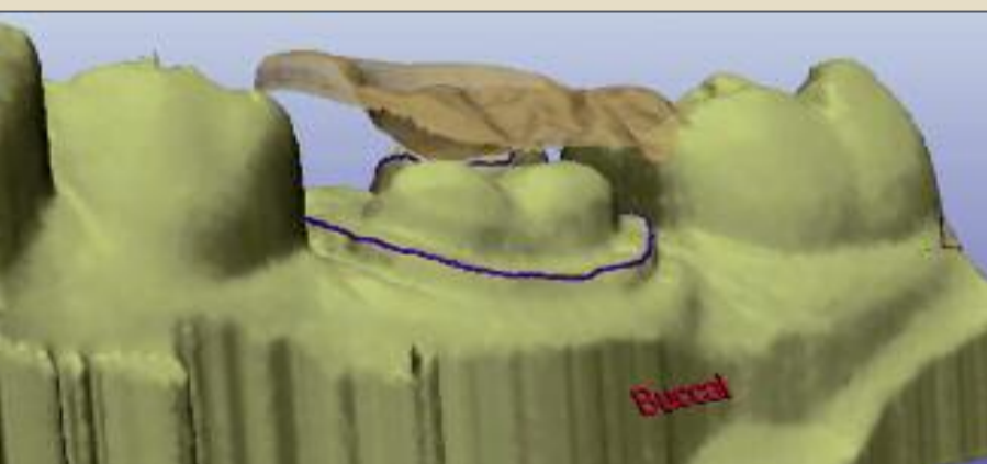
Fig. 1: Virtual automatic reconstruction: the scanned data of the antagonist, functional movement, adjacent teeth and the preparation can be considered in toto, in order to create a fitting occlusal surface that follows all the rules of dentistry and dental engineering. (DTI/Photo A. Mehl)
