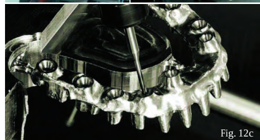
Figs. 12a-c Machining from a titanium block.
