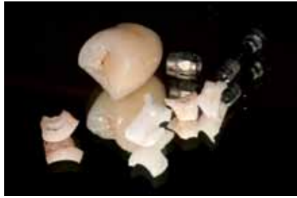
Fig. 2d: The first and the second Procera zirconia abutments were fractured after a short period of service intra-orally.
