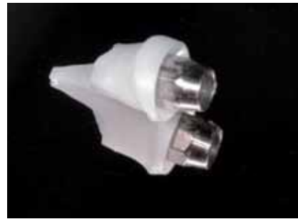
Fig. 3: Digital image demonstrating a fractured zirconia abutment due to over-reduction of the buccal wall.
