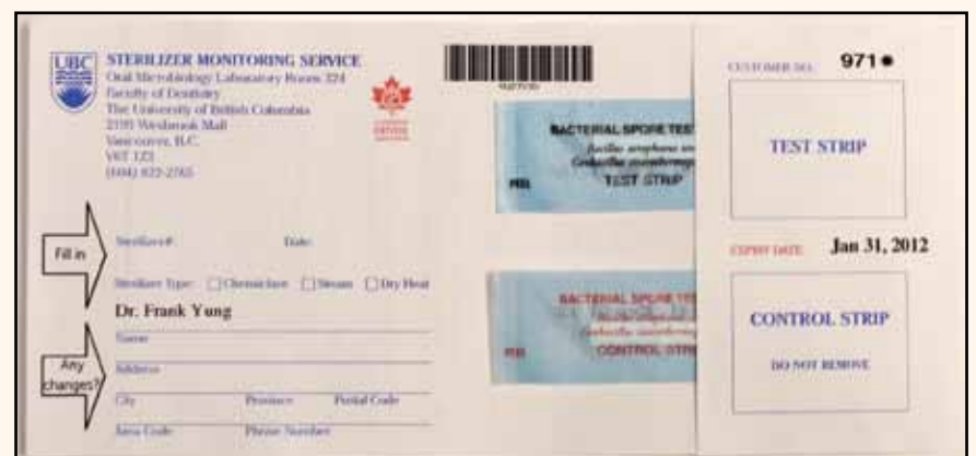
Fig. 2: An example of the submission of indicators to a testing service for assessment of office sterilization equipment's effectiveness.
