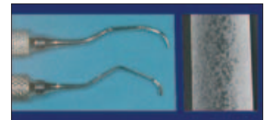
Fig. 7: Alteration of implant surface after use of stainless steel scalers.
