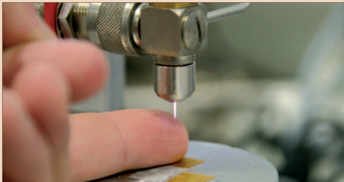
Close-up of a cold plasma jet which is tested under laboratory conditions. (DTI/Photo courtesy of IOM Leipzig)
