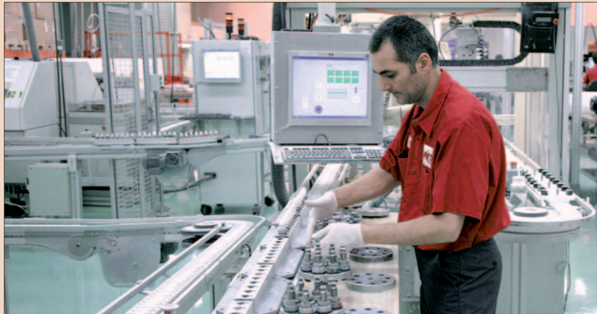
A Nobel Biocare employee prepares the isostatic pressing of NobelProcera crowns. (DTI/Photo courtesy of Nobel Biocare, Sweden)
