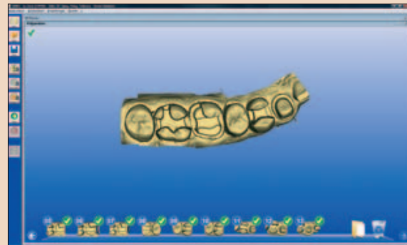
Fig. 2: Quadrant scan with preparations, created from automatically joined individual images to yield a 3-D preview. (Image: Götte)
