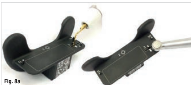
Fig. 8a: Calibration of the drill axis and the instrument tip. Fig. 8b: The Drill-Tag (optical tracking tag).
