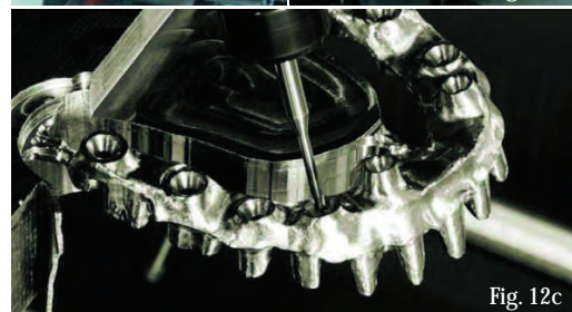
Figs. 12a-c Machining from a titanium block.
