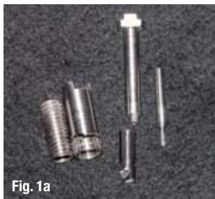
Fig. 1a Components of the bottle-neck device.
