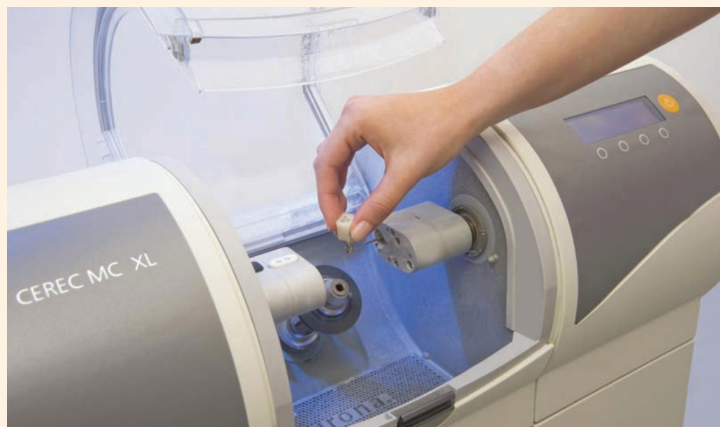
Perfect complements: The CAD/CAM blocks of Sirona and selected partners are optimized to meet the specific requirements of the MC XL milling centers.
