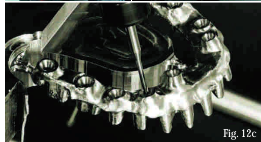
Figs. 12a-c Machining from a titanium block.
