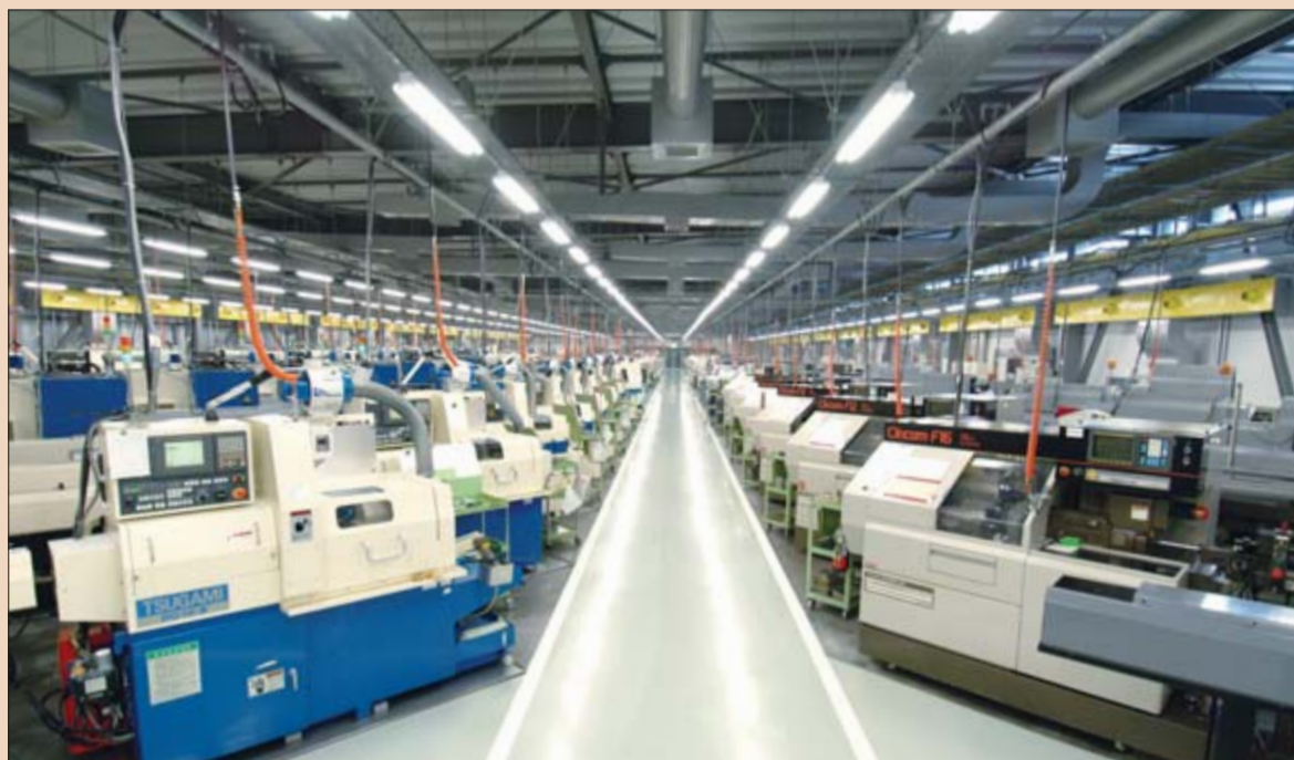
Picture showing production facilities with more than 100 Computerised Numerical Control machines. (DTI/Photo courtesy of NSK Dental, Japan)
