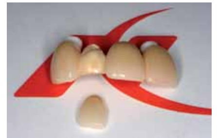
Fig. 4a: Digital image of a broken veneer porcelain from a four-unit, implant-supported fixed partial denture.
