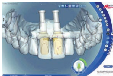
Fig. 5: The Nobel Biocare CAD/CAM software allows ideal screw access site to be planned, then machine fabricated.
