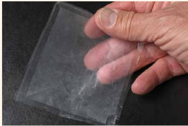
The polymer fibres of which the HelloMask is made produce an apparently transparent membrane but with pores too small for pathogens. (Image: EPFL)
