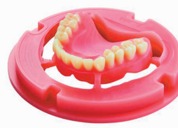
Fig 12: BDLoad, after milling process.
