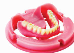
Fig 11: BDLoad, after milling process.
