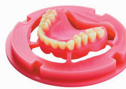
Fig 12: BDLoad, after milling process.
