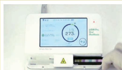
Within 5 minutes, the saliva-testing device produces results regarding the quantity of cavity-causing bacteria and number of white blood cells, for example. Lion Corporation sells the Salivary Multi Test exclusively via a dedicated website.
