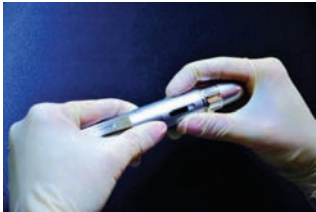
Fig. 3a: Unscrew and remove the cap of the toothbrush.
