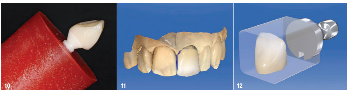
Fig. 10: Specimens embedded in blocks of epoxy resin at angle of 45°. Figs. 11 & 12: Designing of a standardised upper left incisor-shaped crown using CAD-software.
