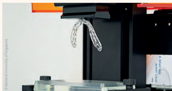
A surgical guide for oral maxillofacial surgery created by a device that uses UV light to cure photosensitive resins into 3-D structures.
