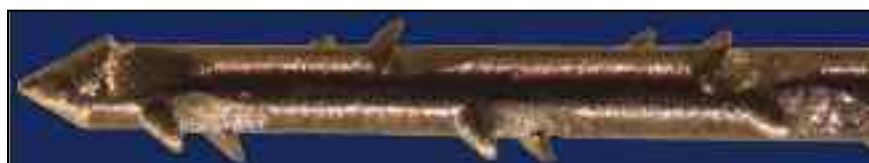
Fig. 4: The broach is formed by forcing a blade onto the surface of a tapered wire.
